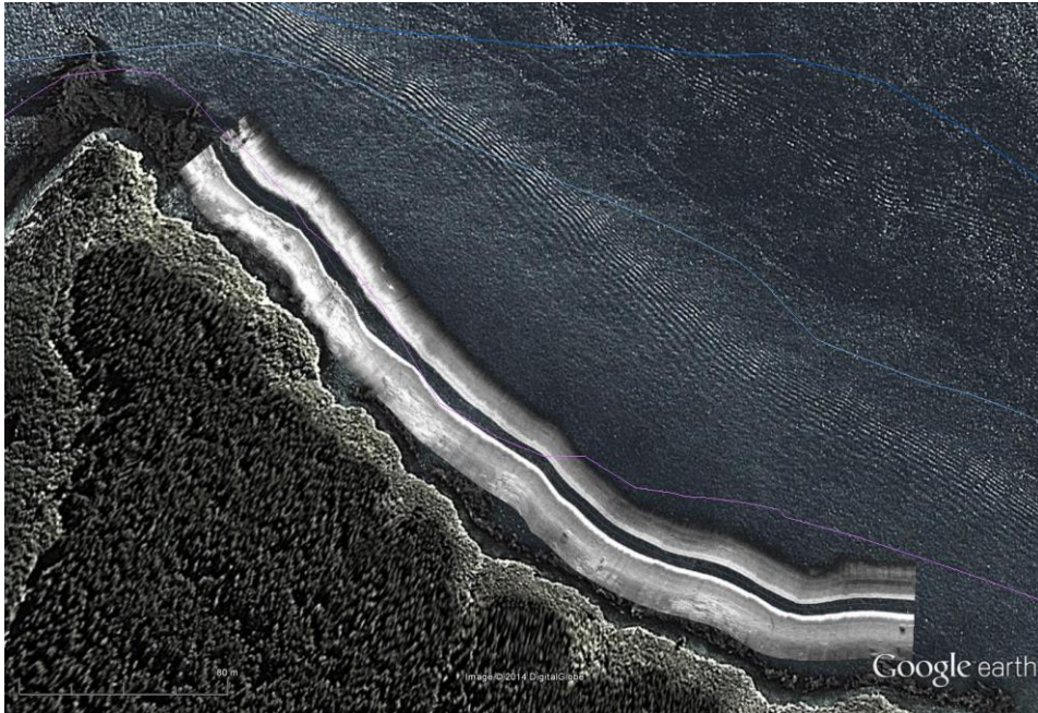
Figure 4-2: Side-scan sonar image (width 60 m) of reef and rocky structures along the shoreline, Oyster Bay. The reef structures lie almost entirely shallower than the 10 m depth contour (pink line).
