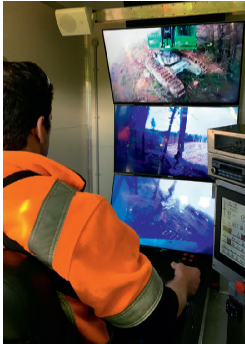
Inside the purpose-built operator's cabin for the tele-operated forest harvester, developed by the Steepland Harvesting PGP programme.
