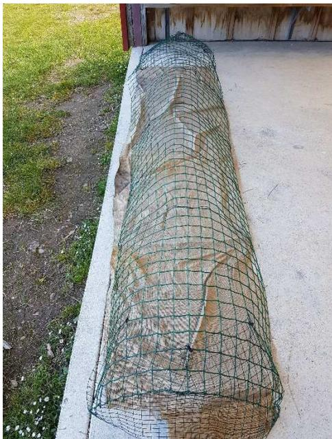
**Figure 3-8: Construction of the exclusion cage with the benthic barrier.**
