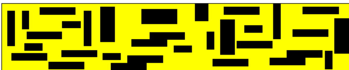
Fouling extent diagram – 30 % localised fouling.
