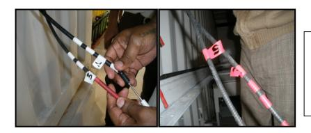
Numbering system to differentiate the house probes in the chamber (white tapes for the right chamber and red tapes for the left chamber). Numbers on the tapes refer to the probe numbers.
