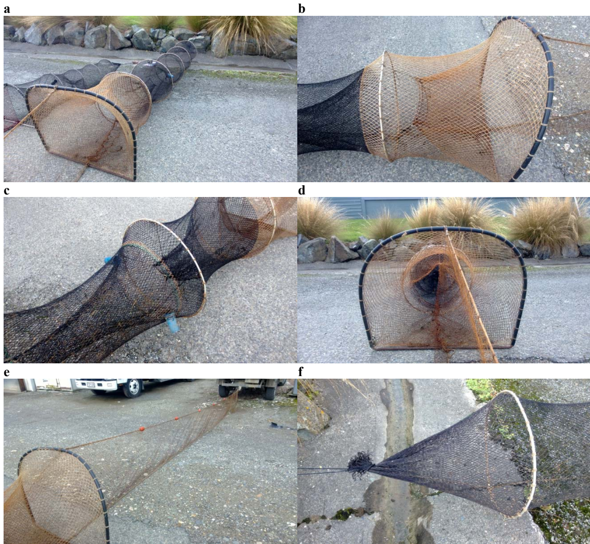
Figure 9: Photographs of a standard South Island shortfin eel fyke net (foreground. a) Full view of net fully extended; b) Net entrance and first valve between the ‘D’ and first hoop. Mesh size between ‘D’ and first hoop is 30 mm reducing to 25 mm thereafter; c) Second and third valves with escape tubes inserted behind the third valve; d) Entrance ‘D’ with leader attachment shown; e) 6 m leader extending away from the ‘D’; f) Codend from which eels are removed from the net. Photos by Mike Beentjes taken at Mossburn Enterprises, Invercargill (February 2014).
